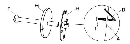
Don't tighten the screws until you have all screws on. Use A-bag screws
